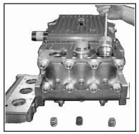
3) Take out pressure springs (57A). Pull out assembled valves (51 & 52) with valve pulling tool (07662).
