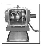
11) Take out plungers and seal sleeves as described above. Drain the oil by taking off the plug (12). After removing the clip ring (33B), pry out the seal retainer (33) with a screwdriver. Remove gear cover (K3).
