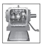
11) Take out plungers and seal sleeves as described above. Drain the oil by taking off the plug (12). After removing the clip ring (33B), lever out the seal retainer (33) with a screwdriver. Open hose adapter (K11) and remove gear cover (K3). Remove the cooling vane plate (K1) by removing the screws (K4)
