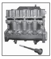
2) Remove discharge casing (50B) up and away.
