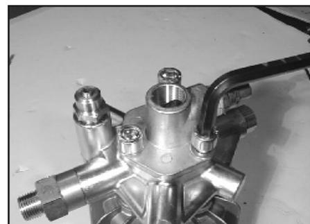
6. Next, remove the three manifold stud nuts (39) with a 17mm wrench. Remove the suction flange (37) and flange o-ring (38). Inspect the o-ring for wear and replace as necessary.
