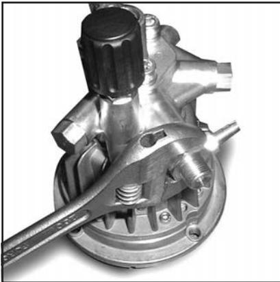
3. With a crescent wrench, remove the injector retainer (76).
