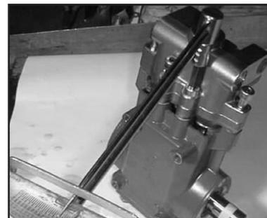
22. Place the valve casing (29) over the plungers. Secure the valve casing with the inner hexagon screws (45). Torque the screws to 36 ft.-lbs (49 NM).
