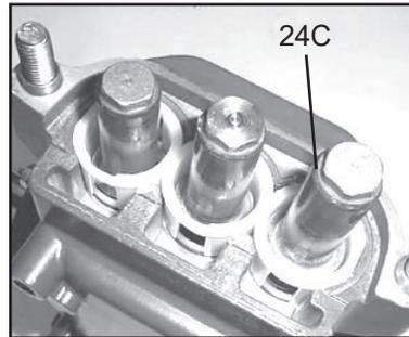
11. Replace copper ring (24C) onto plunger bolt (24B). Slide plunger bolt assembly into ceramic plunger (24A). Apply a light film of loc-tite to plunger bolt threads and place plunger assembly onto stainless steel plunger base (22) and tighten to 200 in.-lbs. (22.5 Nm).
