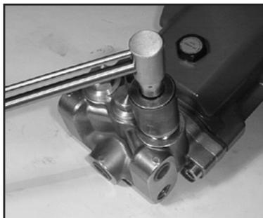
24. Replace the discharge plugs (43) and torque to 52 ft.-lbs (70 NM).
