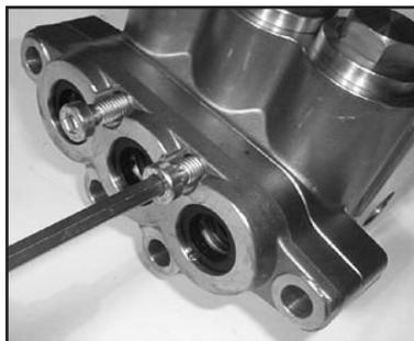
21. Secure the intermediate casing (48) to the valve casing (29) with the inner hexagon screws (46). Torque the screws to 225 in-lbs (25 NM).
