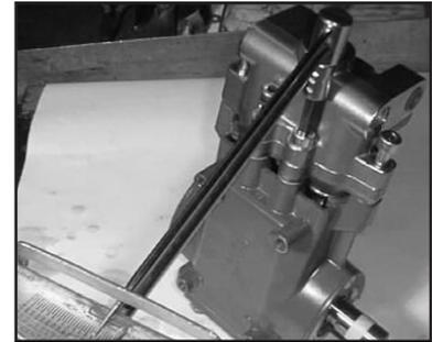
22. Place the valve casing (29) over the plungers. Secure the valve casing with the inner hexagon screws (45). Torque the screws to 36 ft.-lbs (49 NM).
