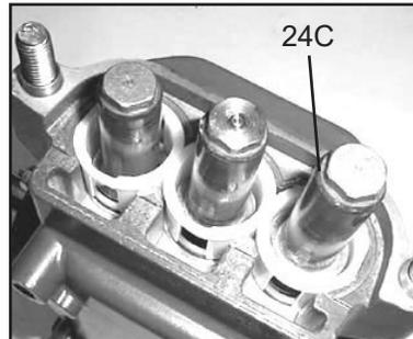
11. Replace copper ring (24C) onto plunger bolt (24B). Slide plunger bolt assembly into ceramic plunger (24A). Apply a light film of loc-tite to plunger bolt threads and place plunger assembly onto stainless steel plunger base (22) and tighten to 199 in.-lbs. (22.5 Nm).
