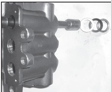
7. Turn the manifold (29) over. Using a 15mm socket, tap out the v-sleeves (31), support rings (32), and pressure rings (30) through back of manifold.
