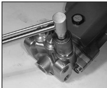
24. Replace the discharge plugs (43) and torque to 51 ft.-lbs (70 NM).
