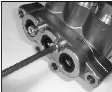
7. Using a 6mm allen wrench, remove the two inner hexagon screws (46).
