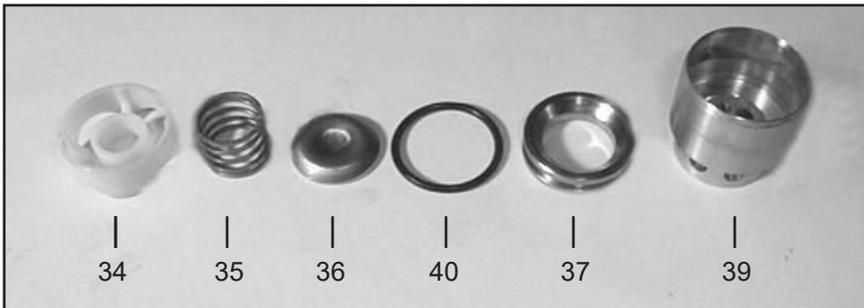
7. Inspect and clean the valve assembly parts. If pitted or worn, replace inlet valve seats (37), valve plates (36), spring (35) and spring retainers (34). Reinsert items 34-38 into valve adapter (39).
