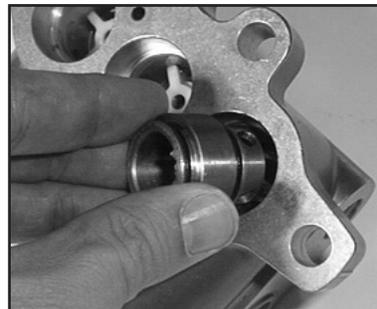
15. Install the seal case (39) with O-rings (40 and/or 40A) into the valve casing (29).
