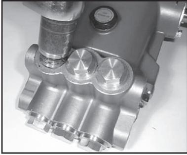
1. With a 22mm socket, remove the three discharge (43) and three inlet (41) manifold plugs. Check o-rings (42 & 44) for wear and replace as necessary.
