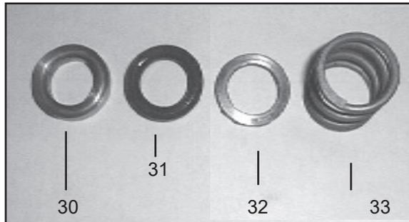
8. Inspect and clean the manifold (29) and pressure ring (32). Reinstall the pressure ring (30) with the grooved side pointed towards the front. Insert v-sleeves (31), support ring (32), and pressure spring (33) into the manifold.
