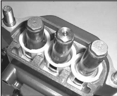
10. Inspect ceramic plunger (24A) tips for wear. If necessary, replacement of the ceramic plungers may be accomplished by removing the plunger bolt assemblies (24B and 24C) with a 13mm wrench. Ceramic plungers should now slide off the stainless steel plunger base (22). Excessive resistance to plunger removal may be overcome by heating the stainless steel plunger base. This will melt any excess loc-tite beneath the ceramic plunger allowing easy removal.
