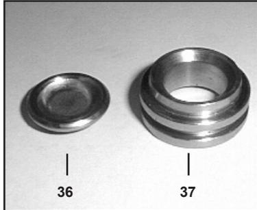
4. Inspect the valve seat (37) and valve plate (36) for signs of wear or cavitation and replace as necessary.
