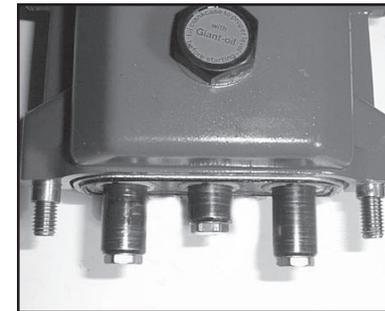
13. Before replacing pump manifold (29), first rotate crankshaft (18) until two outside plungers (24A) extend evenly forward. Next lubricate rear v-sleeves (50) and support ring (51) in the rear v-sleeve housing (48) and slide housing over plungers. Lubricate ceramic plungers with a light film of oil. Carefully and evenly slide manifold over plungers and press manifold firmly against crankcase (1). Replace manifold stud bolts (45), washers (47) and nut (46) and tighten to 35 ft.-lbs. (47.5 Nm).
