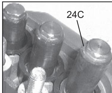
12. Replace copper ring (24C) onto plunger bolt (24B). Slide plunger bolt assembly into ceramic plunger (24A). Apply a light film of loc-tite to plunger bolt threads and place plunger assembly onto stainless steel plunger base (22) and tighten tension screw (24B) to 199 in.-lbs. (22.5 Nm).
