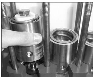
10. Place new plunger pipe (29B) carefully through the oiled seals and push seal sleeve (35) with plunger pipe into the crankcase guide. Reconnect rinsing system.
