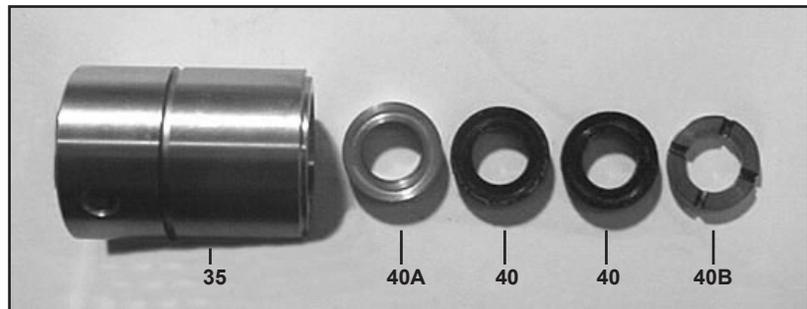
11) Remove the pressure ring (40A), v-sleeves (40), sleeve, and support ring (40B), from the seal sleeve. Remove the pressure spring (41). Examine seals carefully and replace if worn. Clean surfaces of seal sleeves (35) which come in contact with the crankcase (1) and sealing surfaces of valve casing (43).
