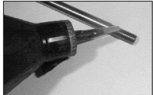
32. Inspect the ceramic plungers (#29B) and replace them if necessary. Clean the ends of the ceramic and remount onto the crosshead/plunger assembly. Make certain that the end of the plunger which is not counter-bored is facing the discharge side of the pump. Install the seal washer (#29D) on the bolt assembly.
