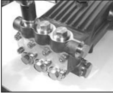
13. Replace plug with O-ring (48, & 48A) and tighten to 107 ft.-lbs. (145 Nm).
