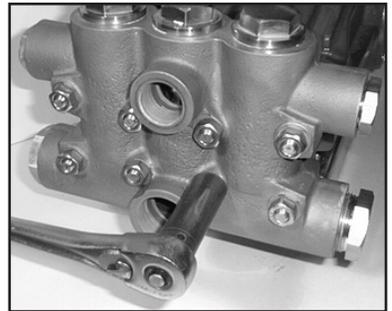
5. Loosen the 8 nuts (49A) with a 19mm wrench. Tap the back of the manifold (43) with a rubber mallet to dislodge and slide off the studs (49).
