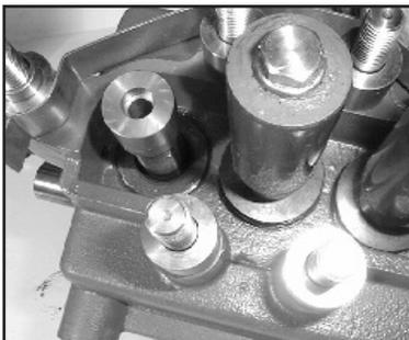
12. Inspect the crankcase oil seals (#31) for evidence of leaking. If there is oil on the crankcase (#1) at the sight of the oil seals, they must be replaced. The oil seals are replaced after removing the crosshead/plunger assembly (#25) as described on page 9.
