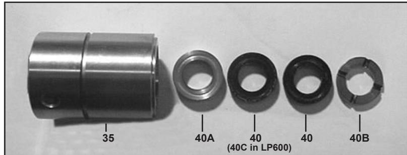
11) Remove the pressure ring (40A), v-sleeves (40), sleeve (40C in LP600 only), and support ring (40B), from the seal sleeve. For LP301A pumps, remove the pressure spring (41). Examine seals carefully and replace if worn. Clean surfaces of seal sleeves (35) which come in contact with the crankcase (1) and sealing surfaces of valve casing (43).
