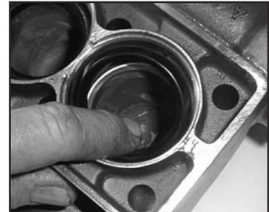
8. Lubricate weep seal (36). Place, weep seal (36), and pressure ring (36A) into the seal sleeve (35). Assemble the O-ring (35A and 35B for LP255 only) onto seal sleeve and lubricate.
