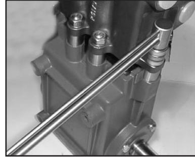
39. Lubricate the plungers (29B) again and slide the manifold (#43) gently and evenly over the plungers. Press the manifold firmly into place against the crankcase (#1). Install the spring washer (#50A) and tighten the manifold stud nuts (#50) to 59 foot-pounds (80 Nm)
