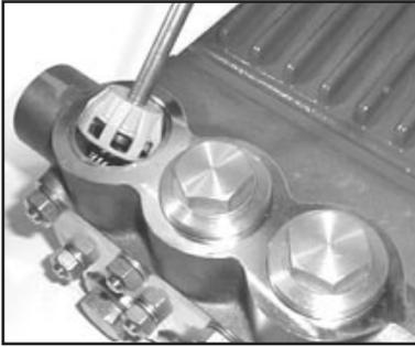
12. Next, place valve assemblies (46A) into manifold after first lubricating the O-ring (44A). Seat firmly into manifold.
