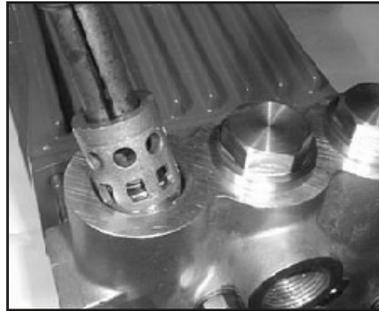
2) Remove discharge and inlet valve assemblies (46) by pulling them upwards out of the valve casing (43). It may be necessary to use a slide hammer tool.
