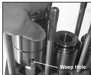
12) Check plunger surface (29B). If plunger pipe is worn out, loosen tension screws (29C) with a 15mm socket and pull off plunger pipe to the front. Clean front surface of plunger (29B) thoroughly. Apply a small drop of loctite to tension screw. Put a **new** crush washer (29D) onto tension screw. Put a thin coat of glue (Loctite) on the ring (or ceramic plunger side) and tighten screw to 265 in.-lbs. (30 NM).
