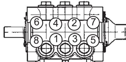
10. Place entire manifold/seal sleeve assembly over the studs and push firmly until seated against the crankcase.
