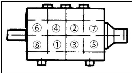
14) Tighten hex nuts (49A) in a crosswise pattern (shown above) to 59 ft.-lbs.
