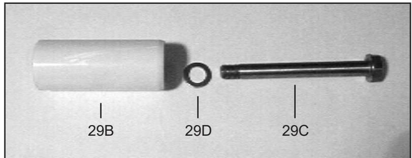
worn, loosen tension screws (29C) and pull off plunger pipe to the front. Clean front surface of plunger (25) thoroughly. Apply a thin coat of Loctite to the tension screw threads (29C). **Note: Care must be taken that no glue gets between the plunger pipe (29B) and the centering sleeve (29A).** Add new copper ring (29D).
