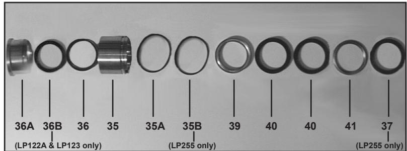
4. Remove the seal sleeve (35) from the manifold and/or crankcase. Remove the pressure rings (39&36A), drip shield (36B for LP122A & LP123 only), v-sleeves (40&36), support ring (41) and O-rings (35A and 35B in LP255A only) from the manifold and seal sleeve, respectively. For LP255 only, remove support ring (37). Examine seals carefully and replace if worn. Clean all parts.
