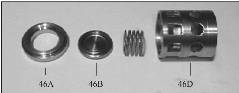
4. Loosen valve seats (46A) from spacer pipe (46D) by lightly hitting the valve plate (46B) with a plastic stick. Check sealing surface and replace worn parts. Reassemble with new o-rings (44A) and oil them before installing. Tighten up tension plugs (48) to 107 ft.-lbs.
