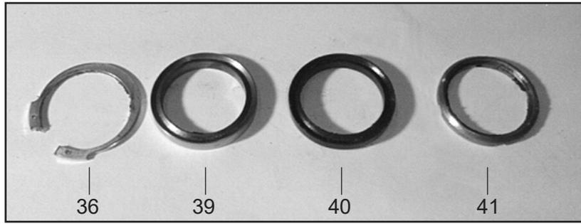
8. From the back of the manifold (#43), remove the packing assembly (#'s 42, 41, 40, and 39) by tapping assembly out from the back to the front.
