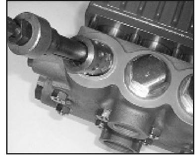
3. Remove the complete valve assembly (46) with valve pullers.
