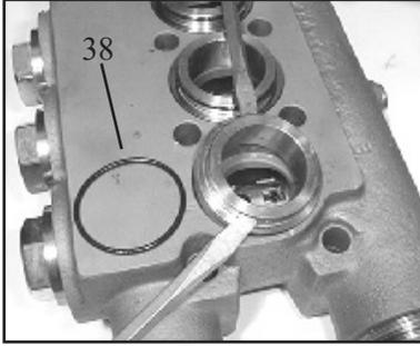
8. Remove seal case (37) from valve casing (43) and inspect o-ring (38).
