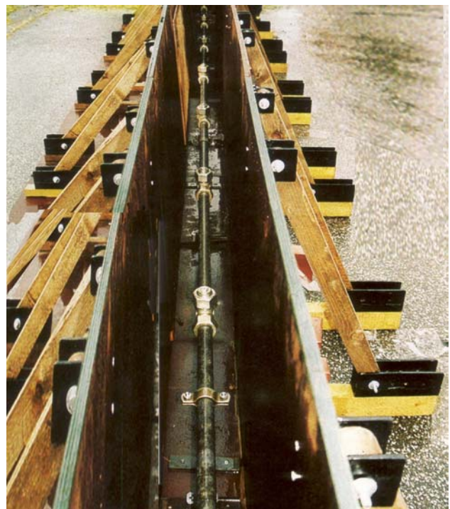
Test Set-up: A provisional construction is used to simulate the function of the Water Safety Wall when sunk into the ground.
