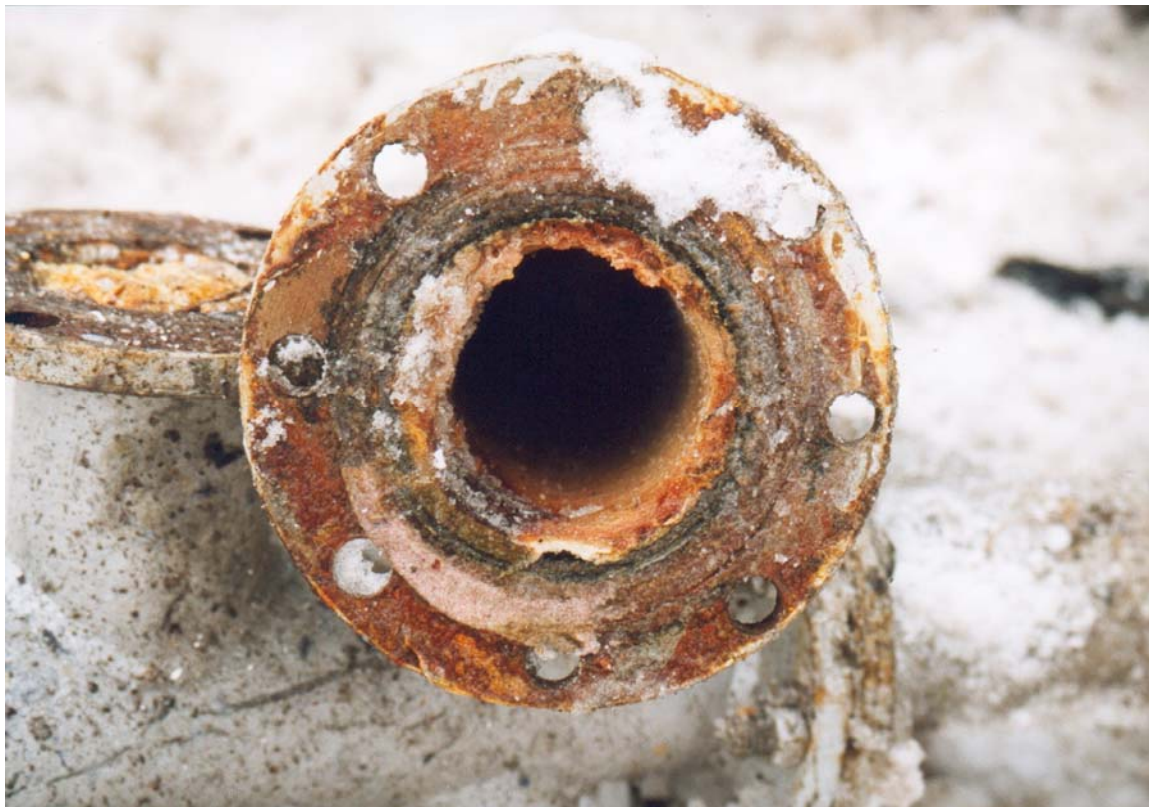
Photo above: The photo shows a pipe ID 100 in use in a plastics factory, blocked with plastic incrustations - prior to cleaning.
