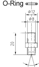
For use with spraying equipment and water tools up to an operating pressure of 21,750 PSI (1500 bar)
