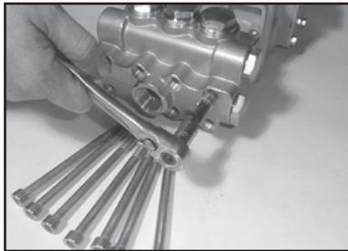
4. Remove hexagon socket screws (34) and remove valve casing (26) by pulling them frontwise over the plungers (16).
