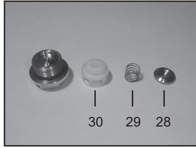
2. Remove the exposed spring tension cap (30) from valve seat by pushing it sideways with a screwdriver. Remove spring tension cap (30), valve spring (29), and valve plate (28).
