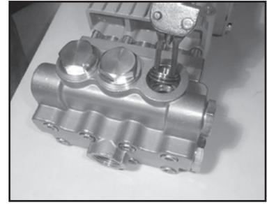
3. Pull out valve seat (27) and O-ring (31) with a valve puller. Check O-ring for wear.
