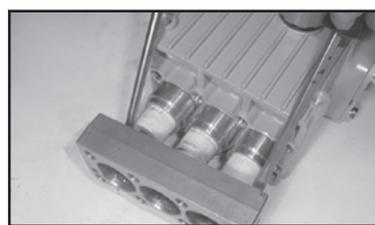
8. Using two screwdrivers, gently pry seal cases (21) out of the valve casing (26) or intermediate casing (25). Press grooved rings (23) and support rings (24) out of intermediate casing (25) using a screwdriver. Check O-rings (21A/25B). Examine seals (23). Replace worn seals.
