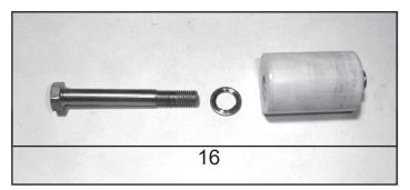
Check plunger surfaces (16). Damaged surfaces lead to accelerated seal wear. Deposits of all kinds must be removed from the plungers.
