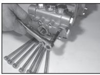
Remove hexagon socket screws (34) and remove valve casing (26) by pulling them frontwise over the plungers (16).
