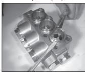
Using two screwdrivers, remove seal case (21) out of the valve casing (26) or intermediate casing (25).
