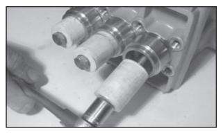
10. If the plunger pipe (16B) is worn, remove tension screw (16D) and remove together with plunger pipe. Check and clean plunger (16A) surfaces and mount new plunger pipe. Cover thread of tension screw (16D) with a thin film of Loctite and tighten carefully at 248 in.-lbs. (28 Nm).
