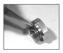
4) Remove the O-ring (31). Inspect all parts for wear and replace as necessary. Apply one drop of loctite 243 to the valve plugs (32) and tighten to 125 lb-ft (170 Nm)
