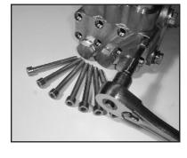
5) Use a 8mm allen wrench to remove the 8 socket head cap screws (34). Carefully slide the valve casing (26) out over the plungers.
