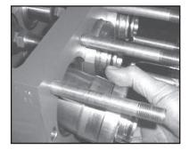
13) Pull seal sleeves (38) and plungers (36) out of their fittings in the crankcase (1) using ring groove as a guide.
