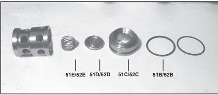
Check surfaces of valve plates (51D and 52D), valve seats (51C or 52C) and o-rings (51B and 52B). Replace worn parts.
