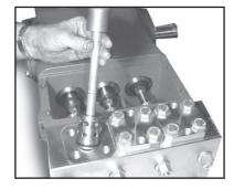
Take out valve assemblies (52 & 51) using either tool (part #07662) or a stud bolt.
