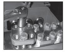
Take plugs (58) out of valve casing (50) by tightening screws (58C) against valve casing with two screws.
