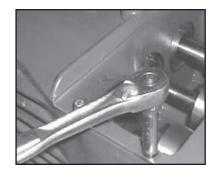
10) Remove cover plate (30) with a 10mm socket wrench.
