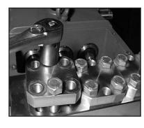
2) Take plugs (58) out of valve casing (50) by tightening screws (58C) against valve casing with two screws.
