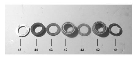
16) Remove support disc (41) seal unit (42, 43, 44) and pressure ring (45) of seal sleeve (38). Examine seals for signs of wear or cavitation, and if necessary, replace.
