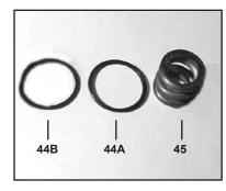
2) Remove the support ring (44B), O-ring (44A) and tension spring (45).
