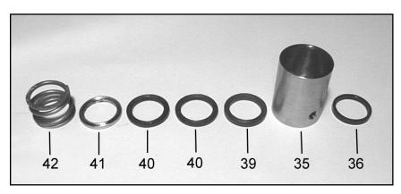
8) Remove the tension spring (42), support ring (41), v-sleeves (40), pressure ring (39), from the seal sleeve (35). Examine seals (36) carefully and replace if worn. Clean all parts.
