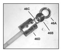
4) Loosen valve seats (46A) and valve spring (46C) from spacer pipe (46D) by lightly hitting the valve plate (46B) with a plastic stick. Check sealing surface and replace worn parts. Reassemble with new O-rings (44A) if possible and oil them before installing.
