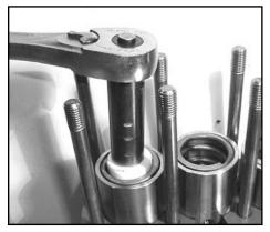
12) Tighten the tension screws (29C) to 26 ft.-lbs. (35NM).The plunger pipe (29B) should not be strained by over tightening of the tension screw (29C) or through damage to the front surface of the plunger; otherwise, it will probably break.
