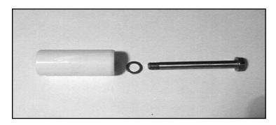
10) Check plunger surface (29B). If plunger pipe is worn, loosen tension screws (29C) and pull off plunger pipe to the front. Clean front surface of plunger (25) thoroughly. Apply a thin coat of Loctite to the tension screw threads (29C). Note: Care must be taken that no glue gets between the plunger pipe (29B) and the centering sleeve (29A). Add new steel ring (29D).
