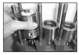
11) Place new plunger pipe (29B) carefully through the oiled seals and push seal sleeve (35) with plunger pipe into the crankcase guide.
