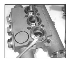
9) Remove seal case (37) from valve casing (43) and inspect O-rings (38/38A).
