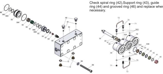
Check surface of plunger (36) for damage. A worn plunger (36) must be removed (27 mm wrench) and replaced. Due to reasons of precision, the ceramic plunger alone cannot be exchanged. Coat the threads of the plunger lightly with an appropriate bonding agent and tighten plunger to the required torque.
