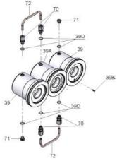
Then push the assembled seal sleeves (39/39A) carefully on to the plungers and into the drive; thereafter, mount elbow pipes (72) as per the exploded view and tighten the screw-in joints (70/71) carefully.
