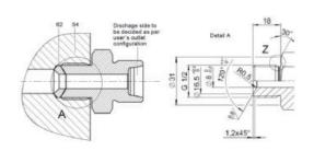
Should a pressure gauge or safety valve be installed, the copper ring (61) must remain in the bore.
