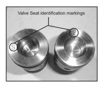
7) When reassembling: The inlet valve seat (51C) is 1mm smaller in diameter than the discharge valve seat (52C). Inlet valve seats are marked "S" and always have to be installed first. Discharge valve seats are marked "P" and are always to be installed on top of inlet valve. Plugs (58) are to be tensioned down evenly with screws (58C) and in crosswise pattern at 155 ft.lbs. (210 N-m).
