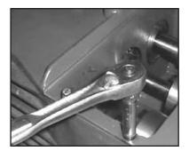
10) Remove cover plate (30) with a 10mm socket wrench.
