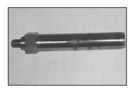
17) Examine plunger (36) for signs of wear or cavitation. If the surface of the plunger is worn, screw out the plunger with a 27mm tool. Clean centering and front surface of crosshead with plunger (25). Thread new plunger carefully through oiled seals in seal sleave. Coat thread of new plunger lightly with bonding agent (e.g., loctite).
