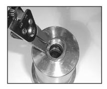
14) Remove circlip ring (48) from seal sleeve (38). Remove spacer disc (47) and seal ring (46) from seal sleeve. Replace worn or damaged parts.
