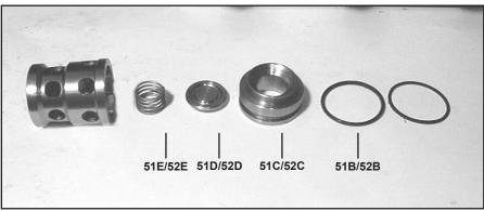
6) Check surfaces of valve plates (51D and 52D), valve seats (51C or 52C) and o-rings (51B and 52B). Replace worn parts.
