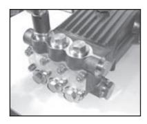
13. Replace plug with O-ring (48, & 48A) and tighten to 107 ft.-lbs. (145 Nm).
