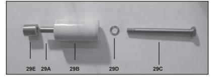
6. Inspect surface of plunger pipe (29B) carefully. Remove any chemical or mineral deposits taking care not to damage the surface of the plunger. If plunger pipe is worn, remove the plunger bolt (29C), plunger pipe (29B) and spacer (29E). Replace worn parts necessary. Note: Always use a new copper gasket (29) when repairing the plunger assembly.
