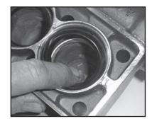
For LP255 pumps, insert support ring (37) into valve casing (43). Place support ring (41) and v-sleeves (40) into valve casing.
