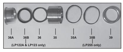
8. Lubricate weep seal (36). Place, weep seal (36), and pressure ring (36A) into the seal sleeve (35). Assemble the O-ring (35A and 35B for LP255 only) onto seal sleeve and lubricate.
