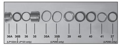
4. Remove the seal sleeve (35) from the manifold and/or crankcase. Remove the pressure rings (39&36A), drip shield (36B for LP122A & LP123 only), v-sleeves (40&36), support ring (41) and O-rings (35A and 35B in LP255A only) from the manifold and seal sleeve, respectively. For LP255 only, remove support ring (37). Examine seals carefully and replace if worn. Clean all parts.
