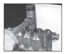
Place entire manifold/seal sleeve assembly over the studs and push firmly until seated against the crankcase.
