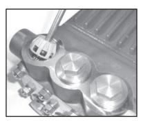
12. Next, place valve assemblies (46A) into manifold after first lubricating the O-ring (44A). Seat firmly into manifold.
