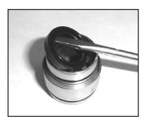
12. Use a 6mm allen wrench to first loosen and remove the tension screw (#16C) from the plunger pipes (#16B). Use a flat screwdriver to pry the oil seals loose from the crankcase (#1).
