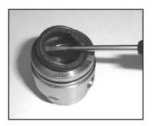
10. Remove the weep grooved seals (#23) from the seal case (#20).
