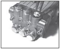
Using a needle nose pliers, remove the inlet and discharge valve assemblies (#32X).
