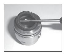
10. Remove the weep grooved seals (#23) from the seal case (#20).
