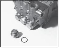
1. With a 24mm socket wrench, remove the (3) discharge valve plugs and (3) inlet valve plugs (#32). Inspect the o-ring (#33) for wear and replace if damaged.
