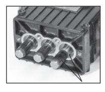
13. Check surfaces of the plunger bases and plunger pipes (#16B). A damaged surface will cause accelerated wear on the seals. Deposits of any kind must be carefully removed from the plunger surface. A damaged plunger must be replaced!
