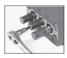
13A. Clean the old sealant from the threads of the tension screw and the plunger base (#16A). Replace the copper washer (#16D). Place plunger pipes over plunger base and secure with tension screw to 200 in.-lbs. (22.5 Nm).
