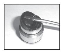
12. Use a 6mm allen wrench to first loosen and remove the tension screw (#16C) from the plunger pipes (#16B). Use a flat screwdriver to pry the oil seals loose from the crankcase (#1).
