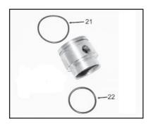
11. Inspect o-rings (#18, #21 and 22) and replace as necessary.
