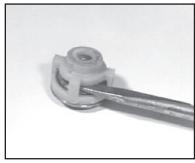
The valve assemblies can be separated by inserting a small screw driver between the valve seat (#27) and its valve spring retainer (#30).
