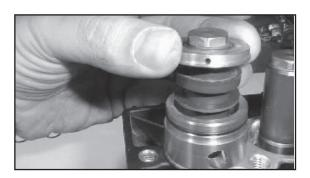
15. Place each seal case (#20) with o-rings (#21, 22) over the plungers (#16). Be certain the oil seal is centered with the seal case and tap firmly until the seal case is seated squarely on the crankcase (#1).
