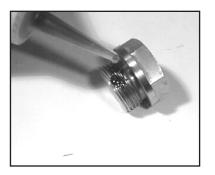
Remove the o-ring (31). Inspect all parts for wear and replace as necessary. For pumps manufactured prior to 5/97, tighten plugs (32) to 33 ft-lbs. otherwise, apply one drop of Loctite 243 to the valve plugs (32) and tighten to 55 ft.-lbs. (75 Nm).
