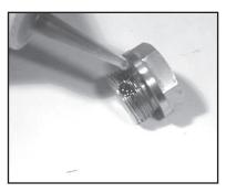
4. Remove the o-ring (31). Inspect all parts for wear and replace as necessary. For pumps manufactured prior to 5/97, tighten plugs (32) to 33 ft-lbs. otherwise, apply one drop of Loctite 243 to the valve plugs (32) and tighten to 55 ft.-lbs. (75 Nm).
