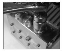
1) Loosen and remove tension plugs (48) with a 36mm socket wrench.
