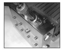
3) Take out discharge valve assemblies (46) by pulling them upwards out of the valve casing (43) with a snap-ring tongs or any other pull-off device. Then remove inlet valves in the same way.
