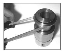
8) Remove seal case (37) from seal sleeve (35).
