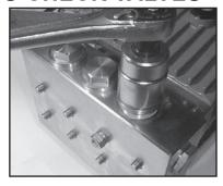
1) Loosen and remove tension plugs (48) with a 36mm socket wrench.
