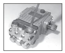
Carefully slide the valve casing (26) out over the plungers.
