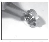
Remove the o-ring (31). Inspect all parts for wear and replace as necessary. Apply one drop of Loctite 243 to the valve plugs (32) and tighten to 55 ft.-lbs. (75 Nm)
