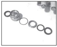
7. Remove the weep return ring (25), pressure ring (24), and v-sleeve (23) from the valve casing (26). Remove the v-sleeve (23A) from the seal case (20). Inspect all parts, including o-ring (21) for wear and replace as necessary
