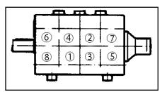
14) Tighten hex nuts (49A) in a crosswise pattern (shown above) to 59 ft.-lbs.
