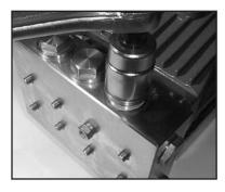
5) Tighten up tension plugs (48) to 107 ft.-lbs. (125 NM)
