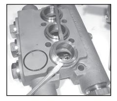
9) Remove seal case (37) from valve casing (43) and inspect O-rings (38/38A).
