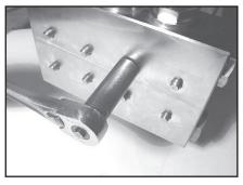
6) Loosen the 8 nuts (49A) with a 19mm socket and pull off valve casing (43) to the front.
