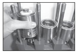
11) Place new plunger pipe (29B) carefully through the oiled seals and push seal sleeve (35) with plunger pipe into the crankcase guide. *Note: Make sure weep hole is facing down.*
