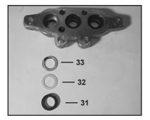
Install the high pressure seal (31) and pressure ring (32) into the intermediate casing (48).
