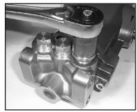
1. With a 22mm socket, remove the three discharge valve plugs (43) from the top of the manifold.
