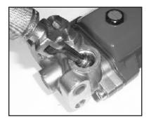
3. Use a slide hammer with a finger attachment to remove the valve seats (37).
