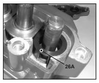
19. Replace the three spacer sleeves (26A) over the plunger with the flanged side toward the valve casing (29).
