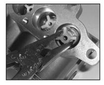
14. Install the inlet valve assembly (34-38) back into the valve casing.
