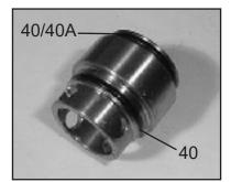
11. Remove the seal case (39) from the valve casing (29) and inspect both o-rings (40 and/or 40A) for wear.
