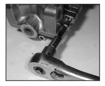
5. Using a 8mm allen wrench, remove the inner hexagon screws (45).
