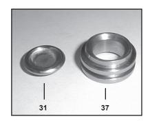
13. Inspect the valve seat (37) and valve plate (36) for wear and cavitation. Replace as needed.
