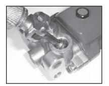
Use a slide hammer with a finger attachment to remove the valve seats (37).
