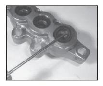
9. Remove and inspect the weep seal (50) and replace if necessary.
