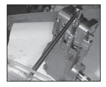
22. Place the valve casing (29) over the plungers. Secure the valve casing with the inner hexagon screws (45). Torque the screws to 33 ft.-lbs (45 NM).
