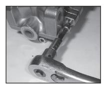
Using a 8mm allen wrench, remove the inner hexagon screws (45).
