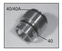
11. Remove the seal case (39) from the valve casing (29) and inspect both o-rings (40 and/or 40A) for wear.
