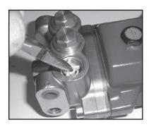
23. Install the three discharge valve assemblies with O-rings (34 - 38).
