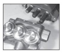
6. With a rubber mallet tap the back of the valve casing (29) and pull the valve casing (29) off the plungers (24A).
