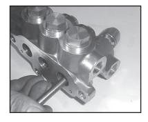
6. From the front inlet valve ports, remove the inlet valve assembly (34-40) and pressure springs (33).
