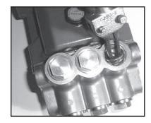
3. Use a small slide hammer to remove valve seats (37) from manifold (29). Inspect valve plates (36) and valve seats (37) for wear. If excessive pitting is seen, replace the worn parts. Check valve seat o-ring (38) for wear and replace as necessary. Tighten manifold plugs (41 and 43) to 52 ft.-lbs. (70 Nm).
