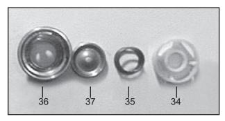
9. If pitted or worn, replace inlet valve seats (36), valve plates (37), springs (35) and spring retainers (34). Re-insert items 34-38 into valve adapter (39). Install valve assembly (34-40) into manifold (29). Reinstall manifold plugs (43) and torque plugs to 52 ft.-lbs. (70 Nm).
