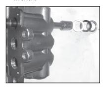
7. Turn the manifold (29) over. Using a 15mm socket, tap out the v-sleeves, Insert v-sleeve (31 & 31A), support rings (32), and pressure rings (30) through back of manifold.
