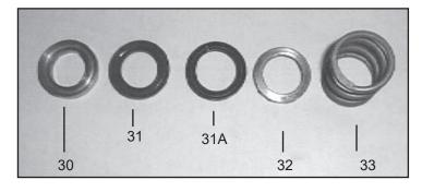
8. Inspect and clean the manifold and pressure ring. Reinstall the pressure ring (30) with the groved side pointed towards the front. Insert v-sleeves (31/31A), support ring (32), and pressure spring (33) into the manifold (29).
