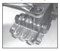
1. With a 22mm socket, remove the three discharge (43) and three inlet (41) manifold plugs. Check o-ring (44) for wear and replace as necessary.
