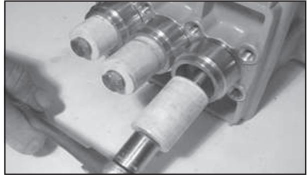
9. Check plunger surfaces (16). Damaged surfaces lead to accelerated seal wear. Deposits of all kinds must be removed from the plungers.
