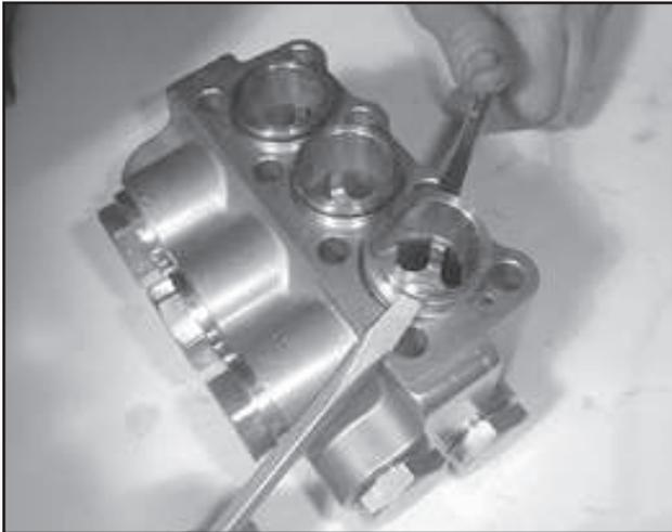
5. Using two screwdrivers, remove seal case (21) out of the valve casing (26) or intermediate casing (25).
