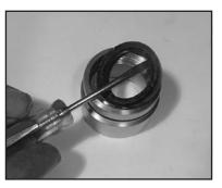
8) Remove the weep grooved seal (23 or 23B) together with pressure ring (24) P420 and P425 only) out of the seal case (20). Check O-rings (21).
