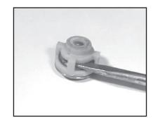
By inserting a small screw driver between the valve seat (27) and the valve spring retainer (30), the valve assembly can be separated.
