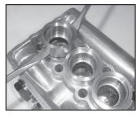
Remove seal case (20) and weep return rings (25) from the valve casing.
