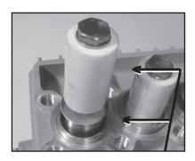
Check surfaces of plunger (16). Damaged surfaces cause accelerated seal wear. Deposits of all kinds must be removed from the plungers.
