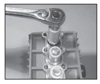
10) If the plunger pipe (16B), is damaged or worn, remove tension screw (16D) and plunger pipe (16B). Check and clean plunger surface (16A) and check flinger (16H). Cover thread of tension screw (16D) with a thin film of Loctite 243 and tighten carefully to 22 ft.-lbs. (30NM).
