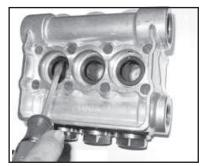
7) Remove the pressure rings (24) and v-sleeves (23 - Note: P422 & P423 pumps have a support ring) from the valve casing (26).
