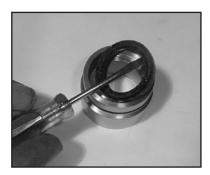
Remove the weep grooved seal (23 or 23B) together with pressure ring (24 -P420 and P425 only) out of the seal case (20). Check O-rings (21). **IMPORTANT!** The grooved seal (23) on the high-pressure side is to be fitted carefully into the valve casing (26) using a screwdriver. Under no circumstances must the seal surface in the valve casing or the seal lip be damaged.
