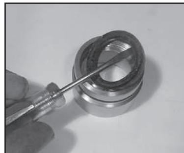
8) Remove the weep grooved seal (23 or 23B) together with pressure ring (24) (P420 and P425 only) out of the seal case (20). Check O-rings (21).
