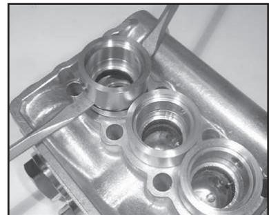
6) Remove seal case (20) and weep return rings (25) from the valve casing.
