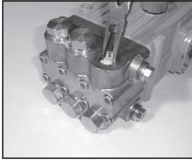
2) Using needle nose pliers, remove the inlet and discharge valve assemblies (27A). Note: It may become necessary to remove the valve seat (27) from the valve casing using a slidehammer.
