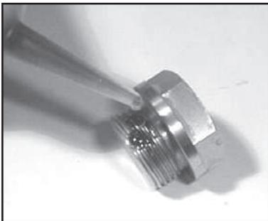
4) Remove the o-ring (31). Inspect all parts for wear and replace as necessary. Apply one drop of loctite 243 to the valve plugs (32) and tighten to 107 ft.-lbs. (145 NM).
