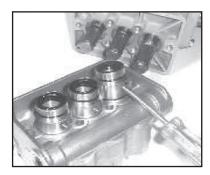
8. Remove weep return rings (#25) from the plungers (#16). Remove the seal case (#20) from either crankcases (#1) or manifold (#26) by using a screwdriver as shown above.
