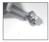
5. Apply one drop of Loctite 243 to valve plugs (#32) and tighten to 55 ft.-lbs. (75 Nm).
