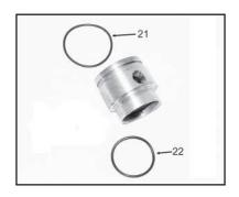
Inspect o-rings (#21 and 22) and replace as necessary.
