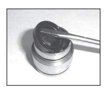
12. For P314, P321 & P327 pumps, use a flat screw driver to pry the oil seals (#19) loose from the seal case (#20).
