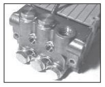
Carefully slide the valve casing (#26) out over the plungers with a screwdriver placed between the valve casing and crankcase.
