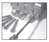
6. Next, use a 6mm allen wrench to remove the 6 hex head cap screws (#34).
