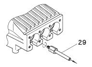
Important! Check the leakage bores ø4 of the seal sleeves (36) and seal cases (46) for dirt and clean if necessary.
