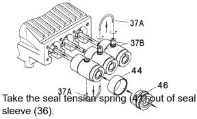
Using a pliers, remove the clip ring (32) situated on the other side of the sleeve; then take out support ring (33) and grooved ring (35) using an extractor tool (either Ø12 or Ø14 - as per plunger Ø).
