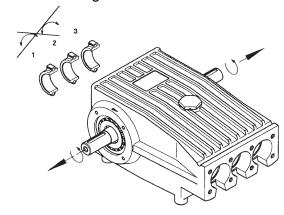
Important! Do not bend connecting rod shafts. Check the running surface of the shaft and connecting rods as well as the shaft seal rings and tapered roller bearings.
