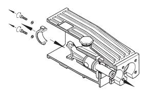
Important! Connecting rods are marked for identification. Do not twist connecting rod halves. When reassembling, connecting rods are to be fitted back onto the shaft journals in their exact original position.
