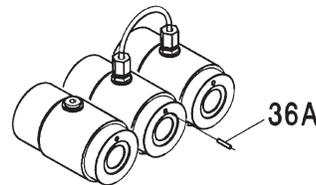
Fit the drip-return unit (32/33/35), the high-pressure seal unit (38, 39, 40) and tension spring (41) into the seal sleeve. Then push the assembled seal sleeves (36) carefully on to the plungers and into the drive; thereafter mount elbow pipes (37A) as per the exploded view and tighten the screw-in joints (37B) carefully. Check O-rings on the drip-return ring (45) as well as border seal ring (43) and replace where necessary.
