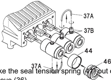
Take the seal tension spring (41) out of seal sleeve (36).
