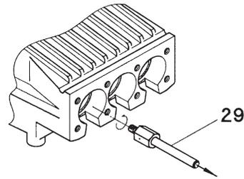
**Important!** Check the leakage bores  $\varnothing 4$  of the seal sleeves (36) and seal cases (46) for dirt and clean if necessary.
