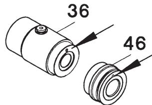
**Important!** The  $\varnothing 4$  leakage bore of the middle seal sleeve must be closed by a rubber plug (36A) to ensure water circulation from seal sleeve 1 to seal sleeve 3.
