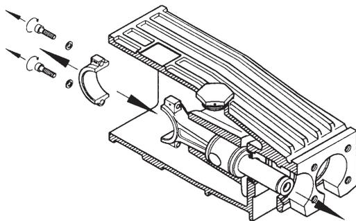
**Important!** Connecting rods are marked for identification. Do not twist connecting rod halves. When reassembling, connecting rods are to be fitted back onto the shaft journals in their exact original position.
