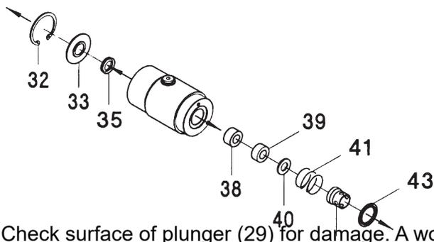
Check surface of plunger (29) for damage. A worn plunger (29) must be screwed out (key size 22) and replaced. Due to reasons of precision, the ceramic plunger alone cannot be exchanged.
