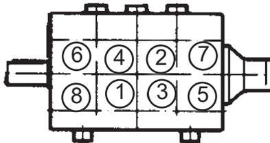
13) Place entire manifold/seal sleeve assembly over the studs and push firmly until seated against the crankcase.
