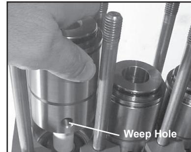
11) Check plunger surface (29B). If plunger pipe is worn out, loosen tension screws (29C) with a 15mm socket and pull off plunger pipe to the front. Clean front surface of plunger (29B) thoroughly. Apply a small drop of locktite to tension screw. Put a **new** crush washer (29D) onto tension screw. Put a thin coat of glue (Loctite) on the ring (or ceramic plunger side) and tighten screw to 22 ft.-lbs. (30 NM).
