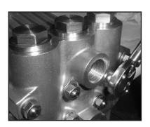
13) Place entire manifold assembly sleeve assembly over the studs (49) and push firmly until seated against the crankcase (1).
