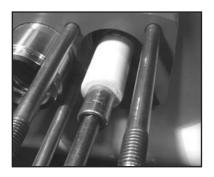
11) If plunger (29B) is worn, remove tension screw (29C) with a 17mm wrench. Clean tension screw with wire brush to remove any old locktite. Discard copper gasket (29D) and replace with new. Clean the front surface of plunger/ crosshead assembly (25). Install new plunger (29B) onto plunger/ crosshead assembly. Put some locktite on both surfaces of copper gasket and tension screw threads. Secure plunger in place with tension screw and gasket and tighten to 26 ft.-lbs. (35 Nm).
