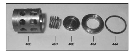
4) Inspect valve seats (46A) and valve plates (46B) for damage and replace if needed. Check valve casing (43) surfaces for damage. Replace O-Rings (44A) and reinstall valve assemblies (46) into valve casing. (Lubricate O-Rings before installation.)
