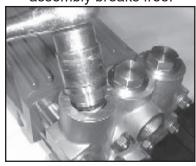
5) Replace tension plugs (48) and tighten them securely to 107 ft-lbs (145 Nm).
