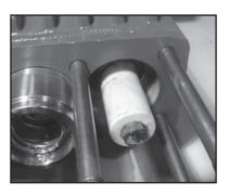
10) Check plunger surface (25 and 29B) and seals (40) for wear and pitting. If none is found, proceed to step twelve.
