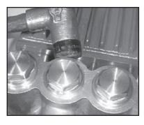
7) If needed, tap valve casing with a rubber mallet to remove it.
