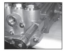
6) Remove the eight (8) manifold nuts and washers (49A,B) using a 19mm wrench and pull off valve casing (43).
