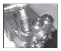
1) With a 30mm wrench remove the three (3) tension plugs (48) along with the tension springs (45) from the top of the valve casing (43).
