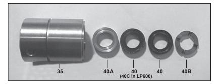
Remove the guide ring (40A), v-sleeves (40/40C), and support ring (40B), from the seal sleeve. Examine seals carefully and replace if worn. Clean surfaces of seal sleeves (35) which come in contact with the crankcase (1) and sealing surfaces of valve casing (43).
