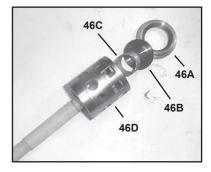
4) Loosen valve seats (46A) valve spring (46C), and valve spring guide (46E) from spacer pipe (46D) by lightly hitting the valve plate (46B) with a plastic stick.Check sealing surface and replace worn parts. Reassemble with new O-rings (44A) if possible and oil them before installing.
