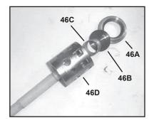
Loosen valve seats (46A) and valve spring (46C) from spacer pipe (46D) by lightly hitting the valve plate (46B) with a plastic stick. Check sealing surface and replace worn parts. Reassemble with new O-rings (44A) if possible and oil them before installing.
