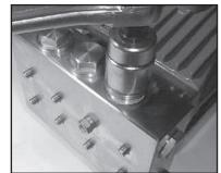
5) Tighten up tension plugs (48) to 107 ft.-lbs. (125 NM)
