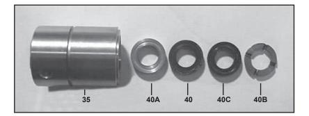
11) Remove the pressure ring (40A), v-sleeves (40/40C), sleeve, and support ring (40B), from the seal sleeve. Remove the pressure spring (41). Examine seals carefully and replace if worn. Clean surfaces of seal sleeves (35) which come in contact with the crankcase (1) and sealing surfaces of valve casing (43).
