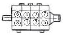
15) Tighten hex nuts (49A) in a crosswise pattern (shown above) to 59 ft.-lbs.
