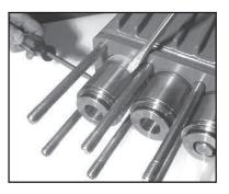
Remove the seal sleeve (35) from the manifold and /or crankcase.
