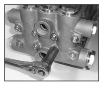
5. Loosen the 8 nuts (49A) with a 19mm wrench. Tap the back of the manifold (43) with a rubber mallet to dislodge and slide off the studs (49).
