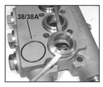
Remove seal case (37) from valve casing (43) and inspect O-rings (38/38A).
