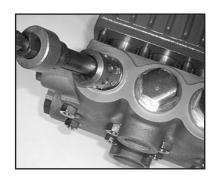
3. Remove the complete valve assembly (46A-46D) with valve pullers.
