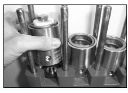
11) Place new plunger pipe (29B) carefully through the oiled seals and push seal sleeve (35) with plunger pipe into the crankcase guide.
