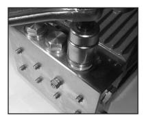
5) Tighten up tension plugs (48) to 59 ft.-lbs. (80 Nm).
