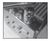
5) Tighten up tension plugs (48) to 59 ft.-lbs. (80 Nm).
