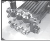
17. Replace plug with O-ring (48, & 48A) and tighten to 107 ft.-lbs. (145 Nm).
