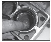
Place support ring (41) and v-sleeves (40) into valve casing. For LP250-3100, the support disc (37) is placed in the manifold (43) before the support ring.
