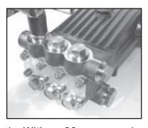
With a 30mm wrench, remove the six (6) plugs (48) from the valve casing (43). Inspect the o-rings (48A) and replace if necessary.
