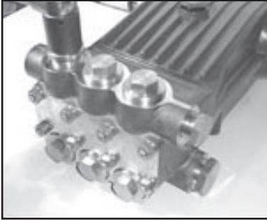
1. With a 30mm wrench, remove the six (6) plugs (48) from the valve casing (43). Inspect the o-rings (48A) and replace if necessary. With needle nose pliers, remove the complete valve assembly (46A).
