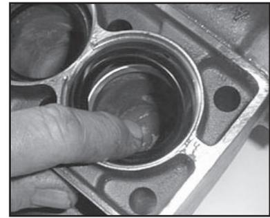
12. Place support ring (41) and v-sleeves (40) into valve casing. For LP250-3100, the support disc (37) is placed in the manifold (43) before the support ring.
