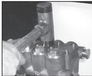
14. Place entire manifold/seal sleeve assembly over the studs (49) and push firmly until seated against the crankcase.
