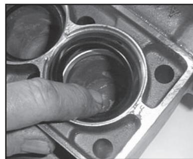
11. Lubricate seal (36). Place seal (36) and drip shield (36B for LP122A-3100 only), and pressure ring (36A) into the seal sleeve (35). Assemble the O-ring (35A) onto seal sleeve and lubricate. LP250-3100 has an additional O-ring (35B).
