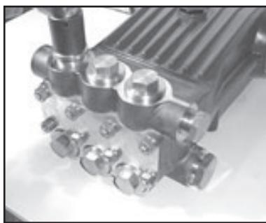
16. Next, place valve assemblies (46A) into manifold after first lubricating the O-ring (44A). Seat firmly into manifold.
