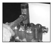
Place entire manifold/seal sleeve assembly over the studs and push firmly until seated against the crankcase.
