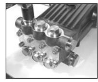
13. Replace plug with O-ring (48, & 48A) and tighten to 160 ft.-lbs. (217 NM).
